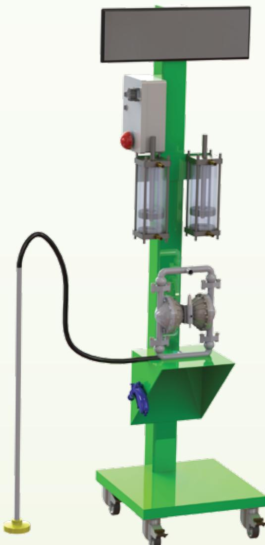
Chemical Dosing System consists of dosage pump, spray gun, dosage unit and hose pipe connection sections. The resin or chemicals with small particles are loaded in the dosage unit and the chemical amount that would be applied onto the garment is adjusted from the unit. With the help of dosage pump, the chemicals are conveyed to the spray gun.
